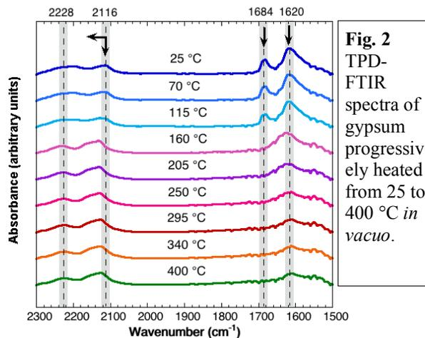
**Fig. 2** TPD-FTIR spectra of gypsum progressively heated from 25 to  $400^\circ\text{C}$  *in vacuo*.
