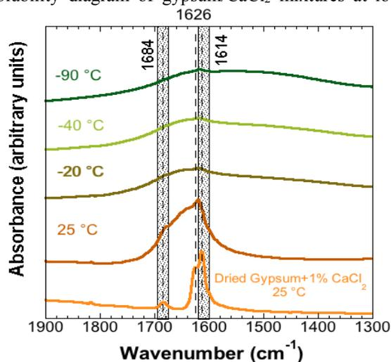
**Fig. 3** Cryogenic-FTIR spectra of the gypsum+1%  $\text{CaCl}_2$  mixture in the H-O-H bending region.
