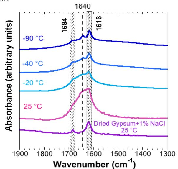
**Fig. 4** Cryogenic-FTIR spectra of the gypsum+1% NaCl mixture in the H-O-H bending region.
