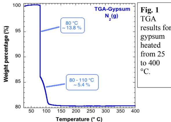
**Fig. 1** TGA results for gypsum heated from 25 to  $400^\circ\text{C}$ .
