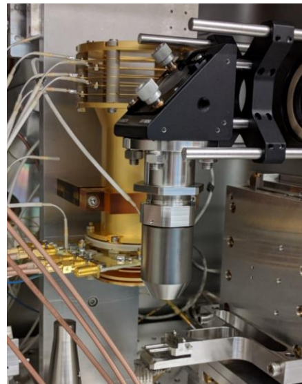
Fig. 1 Miniature mass analyzer (in gold) and high-resolution microscope system (in grey). The mass analyzer has a dimension of 160 mm x Ø 60 mm. Combined, they enable chemical context analysis of solids.
