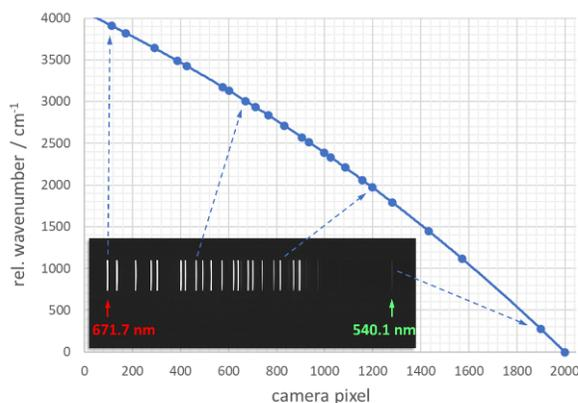
**Figure 2:** Spectral calibration of the BBM with a Ne lamp in the range of 0 to  $4000 \text{ cm}^{-1}$ . Inset: Raw detector image with the individual slit images.
