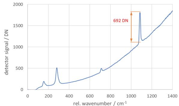
**Figure 4:** Raman spectrum of calcite. The  $1086 \text{ cm}^{-1}$  line achieves an SNR of  $> 800$  (exposure time: 60s).
