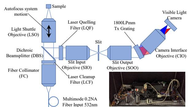
**Figure 1:** Scheme of the RAX optical system. Inset: Picture of the RAX BBM at DLR-OS.
