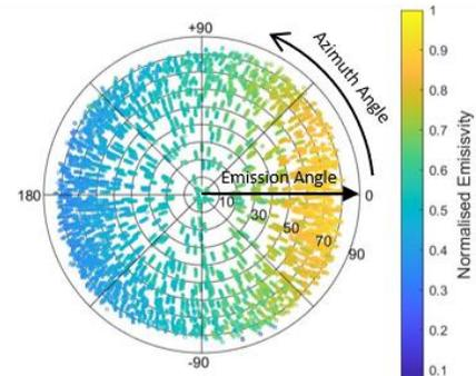
**Figure 2:** Diviner-measured EPF at  $70^\circ$  incidence angle for the high-latitude highland target.
