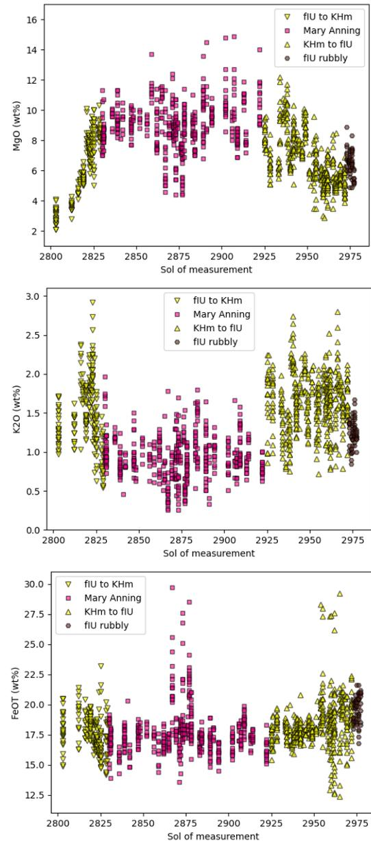
▲ **Figure 2:** variations in MgO, K<sub>2</sub>O and FeO<sub>T</sub> abundances (wt%) along the traverse. The x axis shows time of measurement and does not reflect horizontal distance. The diagrams start just after the departure from Bloodstone Hill and ends at the Sands of Forvie (see Figure 1 for localization of the rover stops). Each symbol corresponds to a single LIBS point on a bedrock target, excluding Ca-sulfate veins and soils.
