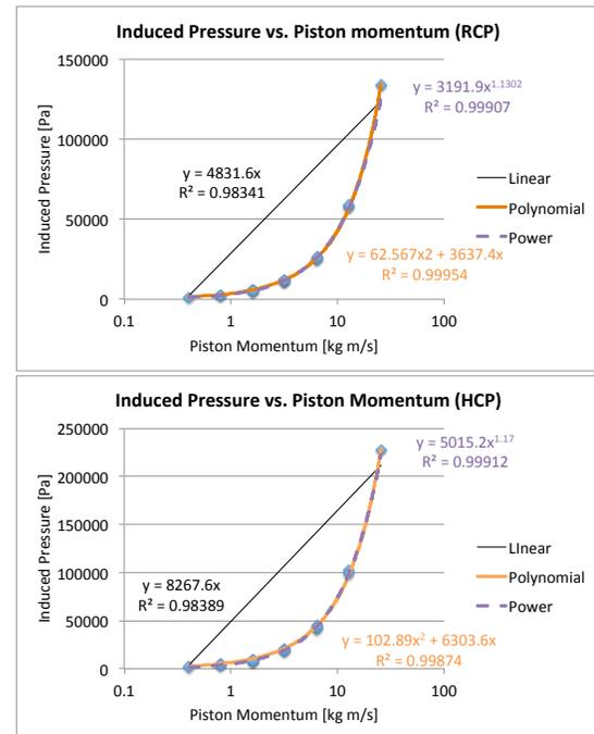
Figure 2: Wave-induced pressure vs. piston momentum for the RCP and HCP configurations. Three different trend lines have been included as well as their equations.
