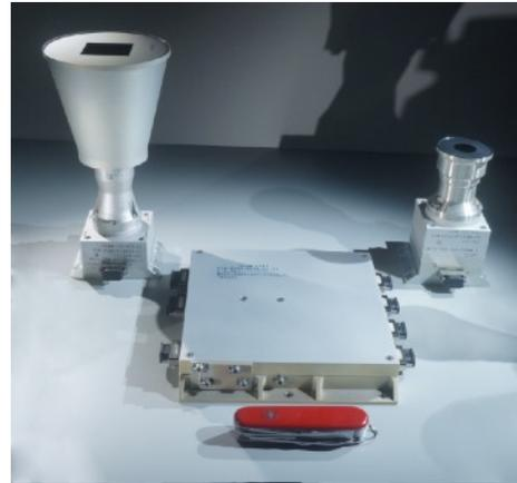
Figure 3: A Mailin Space Science Systems ECAM-M50 (Monochrome) with NFOV (Narrow Field of View) lens (left), ECAM-IR3 (right), and ECAM-DVR4 (center). JCam will appear similar to this shown flight camera system with different lenses. Pocket knife for scale. Credit Malin Space Science Systems.
