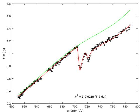
Figure 1: (Red curve) Best fit to (Fe carbide, sulfide, silicate) standard set. Green curve: assumed background, using a third-order polynomial fit to the continuum below the Fe L-edge.
