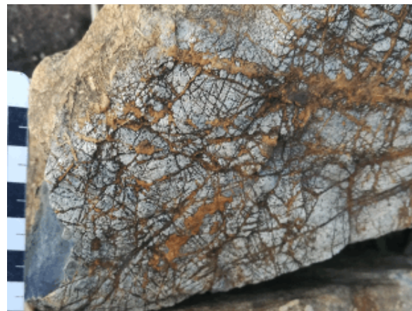
Figure 3: In situ brecciated basalt, with carbonate veins.
