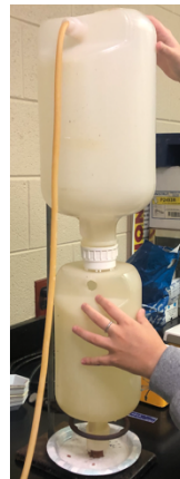
Figure 1. The bottle method used to perform compression strength tests. The bottle is filled using a tube connected to the top of the bottle. The sample is under the bottom of the stacked bottles.
