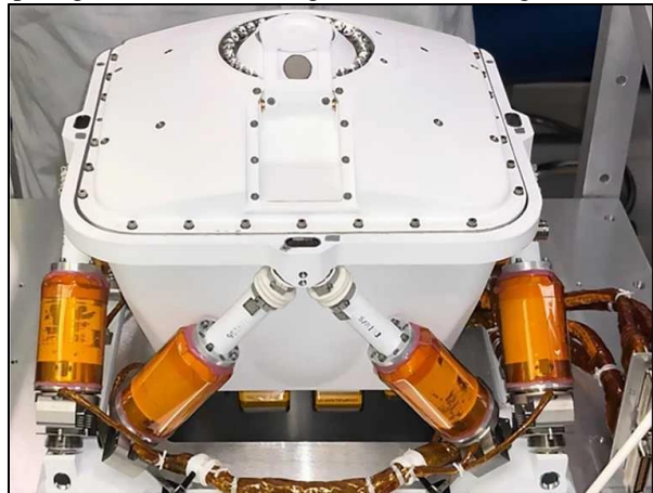
Fig. 1: The PIXL sensor assembly prior to integration on the rover arm turret.
