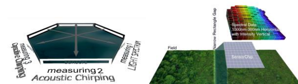
Fig. 4. Remote sensing: A Full Spectrum Scanner Field Scanning. A narrow gap with a prism and a CCD on which the full spectrum is mapped.
