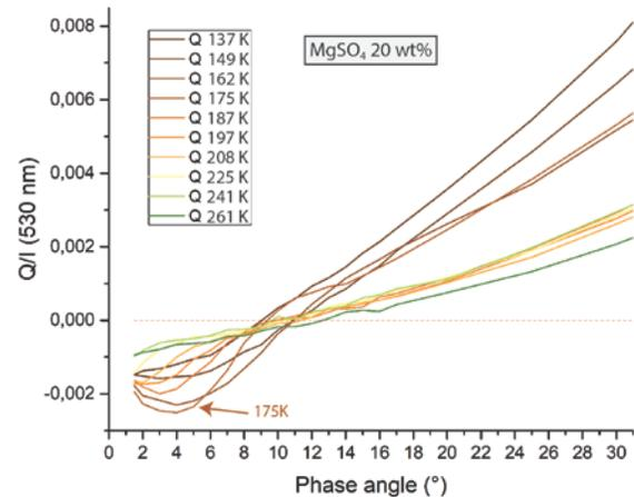
Figure 2: Polarimetric phase curves of flash-frozen icy particles made from a liquid solution of 20 wt% of  $\text{MgSO}_4$ .
