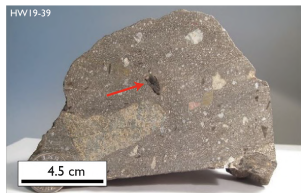
Fig. 2. Cut surface of polymict lithic impact breccia (sample HW19-39) with organic fragments (red arrow) and carbonate melt clasts.
