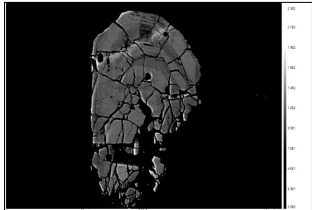
Fig 1: BSE image of compositionally zoned and highly fractured zircon grain from suevite breccia. Note that the near subhedral grain is ‘digested’ in the lower right corner.
