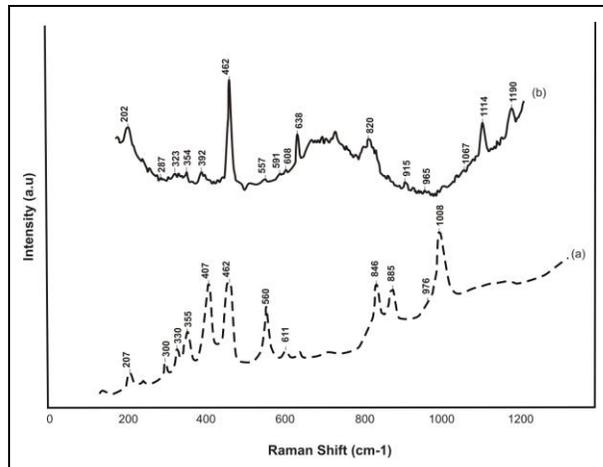
Fig 2. Raman spectra of reidite bearing zircon from Dhala structure (b) within a grain of ballen quartz. The data is compared with that of reidite bearing Zircon from Xiuyan crater [6]. Raman peaks at 287, 323, 392, 462, 557, 591, 608, 638, 820, 915, 965, 1067, 1114, 1190  $\text{cm}^{-1}$  are attributed to reidite (b).
