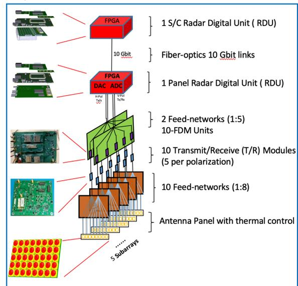
**Fig. 2:** SESAR is modular instrument approach consisting of “smart panels” made up of lightweight antenna elements and power-efficient radar electronics. This approach enables the same design to be scaled to match the science goals and orbit of different planetary targets.
