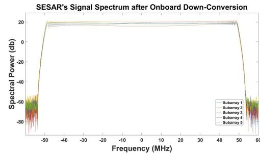
**Fig. 4:** RDU's firmware and hardware functionality demonstration in the laboratory. The five 100-MHz bandwidth (baseband) waveforms correspond to SESAR's single panel FDM waveform generation and data acquisition obtained with the RDU in transmit-receive loopback configuration.
