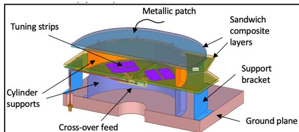
**Fig. 3:** Cross section of one antenna element with the composite design. We are currently building test elements to validate the design; a full SESAR panel is 5 x 8 of these elements.
