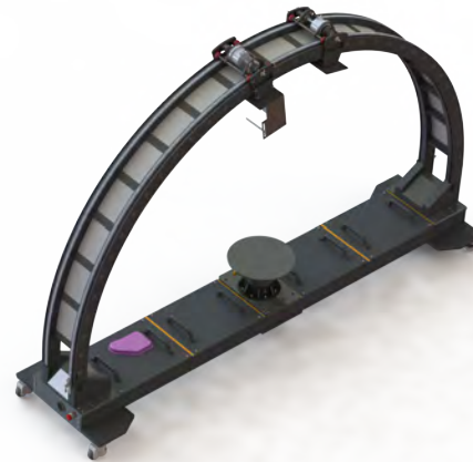
Fig. 2. CAD rendering of the PSTL goniometer. Samples are placed on the circular stage at the center of the base. Caddies for the light source and camera are shown at the top of the arc.
