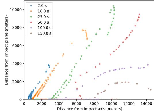
*Figure 2 - Ejecta curtains at different times on Earth. The points on this graph are the tracer particles showing the leading and trailing edges of the ejecta cloud. Each color corresponds to a different time in the simulation. The crater and injection cells are in the bottom left corner of the graph. Note that this figure has a different vertical scale as compared with Fig. 1.*
