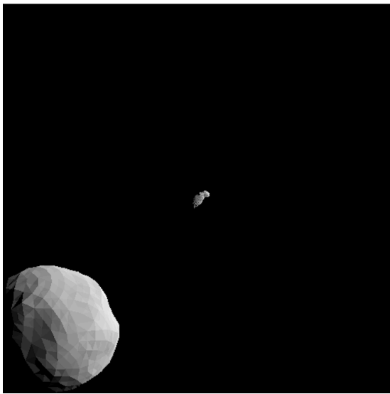
Fig. 1: Simulated view of the DRACO camera 129 seconds before impact. The shape used for Dimorphos is asteroid Itokawa, reduced in size to match the real dimensions.
