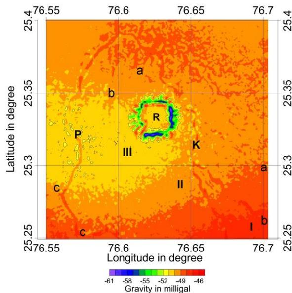
Figure 2. Satellite Bouguer gravity map of RC (R) and surrounding area, abbreviations: aa, bb, cc- NW-SE gravity lineaments, I (less than -48 mGal), II (-50 to -48 mGal) and III (-51 to 50 mGal) are areas of different Bouguer gravity, P- Parvati River, K- Kul River.
