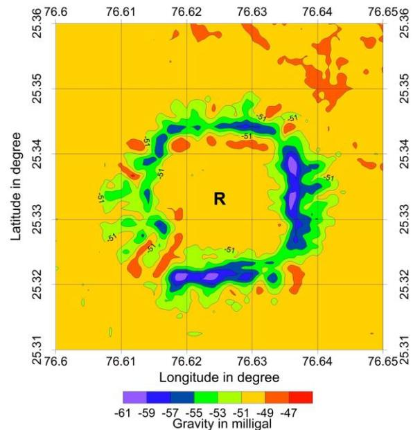
Figure 3. Satellite Bouguer gravity map close to RC, note the lowest values of gravity anomaly (-61 to -59 mGal) are observed only along the visible rim of the crater.
