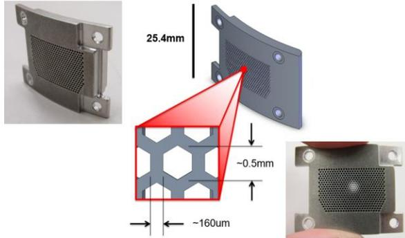
FIGURE 3: FINAL COLLIMATOR DESIGN
