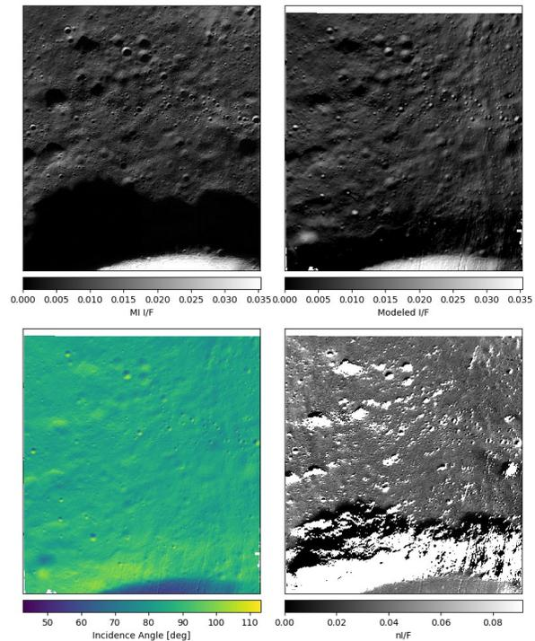
**Figure 4.** Sample MI image (ID: 03\_04747S848E1173) in  $I/F$  (upper left), modeled  $I/F$  derived by Hapke model (upper right), incidence angle layer (lower left), and  $nI/F$  (lower right). Southern rim of Idel’son L crater is shown in the bottom of all images. In the bottom right panel, the dark zone above the shadowed region (white null pixels) corresponds to abnormal  $nI/F$  area, caused by the unpredicted shadow.
