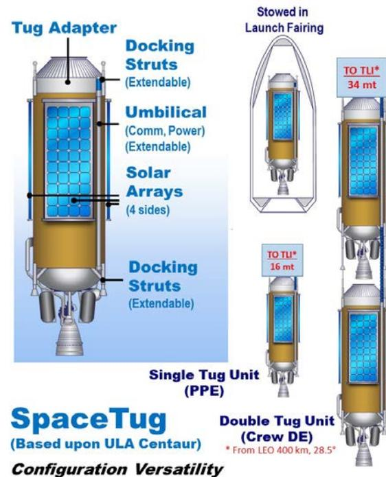
Figure 1: SpaceTug Configurations
