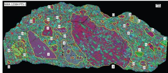
**Figure 1.** AlMgFe X-ray map of PTS-1 with clast outlines. The quantitative compositional map is of basalt clast 3.
