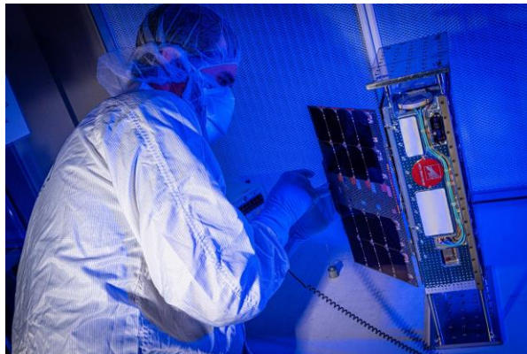
Figure 1. A Ball Aerospace technician stows the solar panels on CIRiS to complete the final assembly before shipment on September 25 th , 2019.
