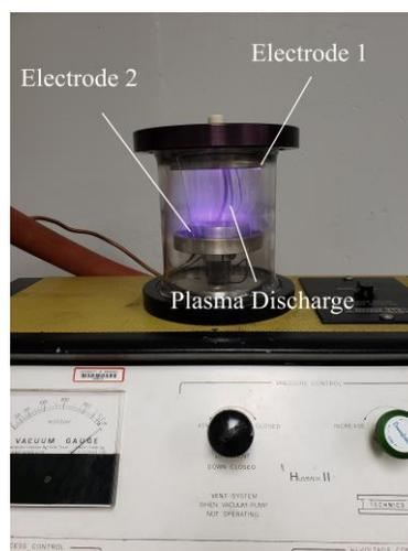
**Figure 1:** Technics Hummer II sputtering chamber (housed at the Arkansas Center for Space and Planetary Sciences) triggering a DC cold plasma discharge at 30mA that ionizes the Titan-simulated N<sub>2</sub>-CH<sub>4</sub> (90%-10%) gas mixture to produce tholins after several days.
