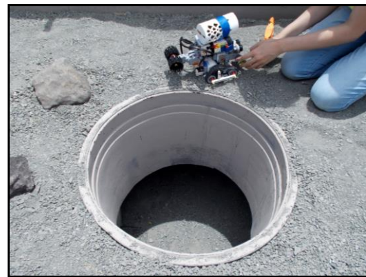
Figure 2. Simulant test bed with modeled lunar sky-light and student robot with attached CanSat.
