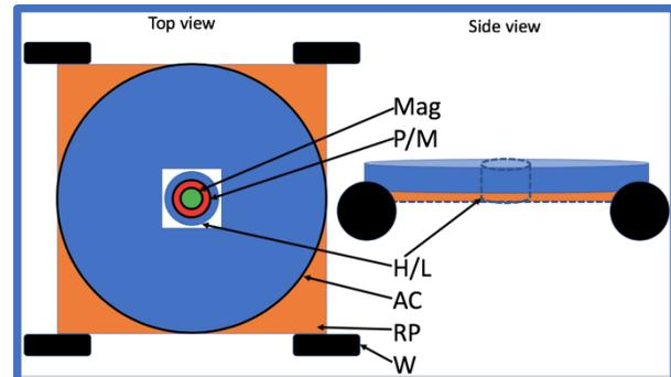
Fig. 1: components are shown above: Mag – Magnetometer, P/M – Pulse/Magnet, H/L Heater/Laser, AC – Alternating current Coil, RP – Rover Platform, W – Rover's Wheel. Wheels are about 1 m apart.
