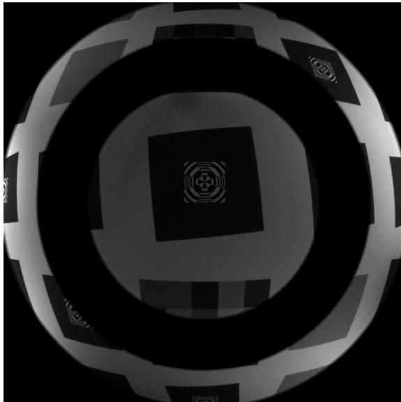
Figure 3. SkyCam image of geometric calibration target.
