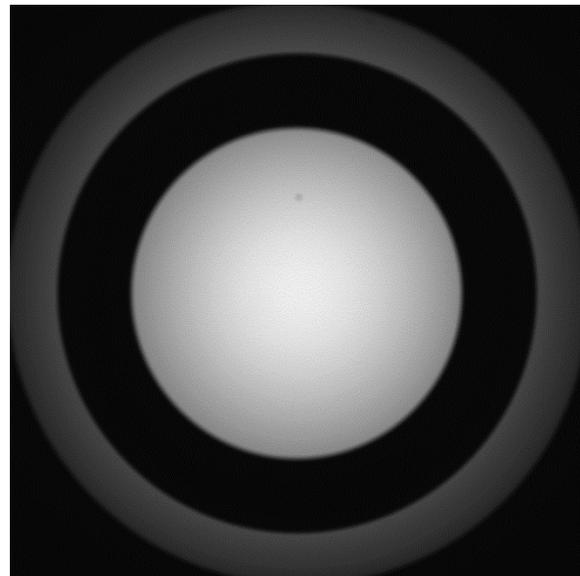
Figure 2. SkyCam flat field image. This image shows the characteristic response fall off of fisheye lenses; a circular region centered on the rover zenith; an annulus of reflective neutral density 5 material for solar flux measurements; an annulus that will show sky light to >60° from zenith; and the circular baffle in the corners.
