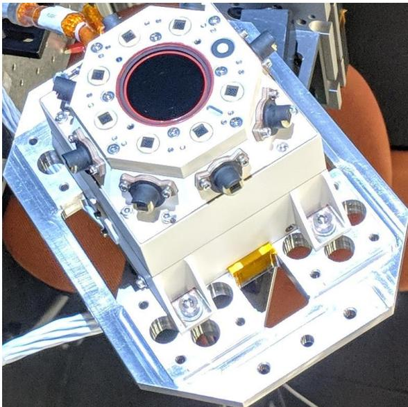
Figure 1. The RDS assembly. The SkyCam window is the dark circle in the center of the top plate.
