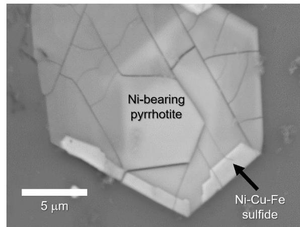
**Figure 1.** Electron backscattered (BSE) photomicrograph of an Fe-sulfide assemblage exposed on the wall of a vesicle in Pica glass. The rim appears similar to overgrowths of cubanite (CuFe<sub>2</sub>S<sub>3</sub>) observed on Fe-sulfides from CI meteorites, Stardust samples from Comet 81P/Wild, and experimentally produced sulfides prepared in environments intended to simulate aqueous alteration on comets [9-11].
