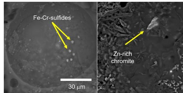
**Figure 4.** Electron backscattered (BSE) photomicrographs of an Fe-Cr-sulfide grains and a Zn-rich chromite grain exposed in vesicle walls in Edeowie glass.
