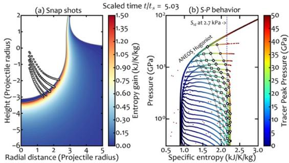
**Figure 2.** (a) Snap shot at  $t = 5 t_s$ ,  $v_{\text{imp}} = 4.14$  km/s and  $Y_{\text{lim}} = 0.65$  GPa. The color map means the entropy gain. (b) The thermodynamic track on a entropy-pressure plane. The color indicates the peak pressures of tracer particles.
