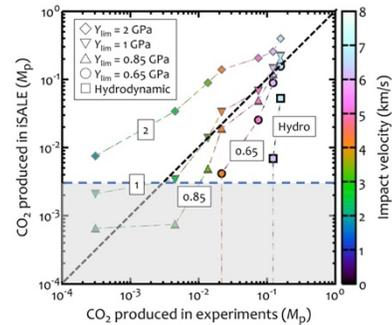
**Figure 3.**  $M_{\text{CO}_2, \text{exp}}$  vs  $M_{\text{CO}_2, \text{calc}}$ . The color bar indicates impact velocity.
