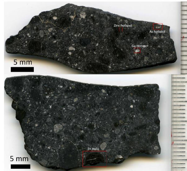
Figure 1. Visible light maps of slabs of NWA 8171, a typical sample of Martian regolith breccia meteorite consisting of a wide variety of lithic clasts. Four regions of interest are highlighted.
