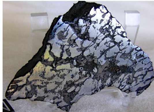
Fig. 2. Slice of the IAB complex iron Georgetown showing troilite dendrites (brown) in metallic Fe,Ni (white). Photo courtesy of Anne Black, Impactika.
