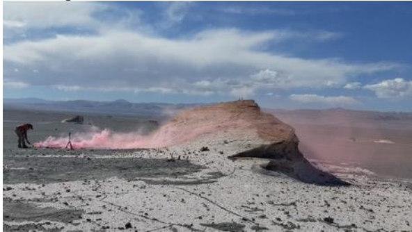
Figure 3. Flow visualization using smoke tracers showed an alignment between the observed secondary wind direction, dedos, and a facet cut in the back of the yardangs in the areas.
