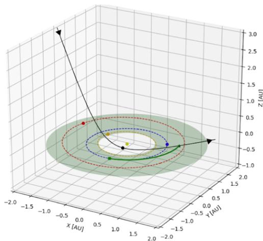
**Figure 2:** Example mission trajectory to 1I/Oumuamua had Bridge been launched on 6/27/2017 and intercepted on 10/22/2017. The solid black line is 1I/Oumuamua, and the solid green line is the Bridge spacecraft. Total flight time would have been 116.85 days, and resulted in a relative intercept velocity of 55.97 km/s.
