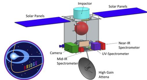
**Figure 1:** Bridge spacecraft conceptual design including all instruments.
