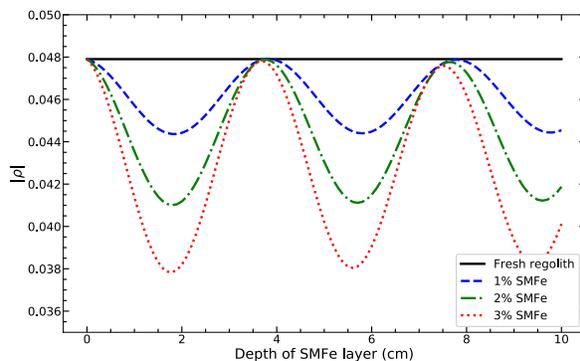
**Figure 2:** Reflectivity of the two-layer model with varying SMFe volume fraction and depth of the upper weathered layer.
