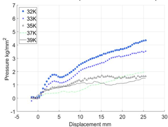
**Figure 2: Pressure versus indenter penetration depth curves for various temperatures.**
