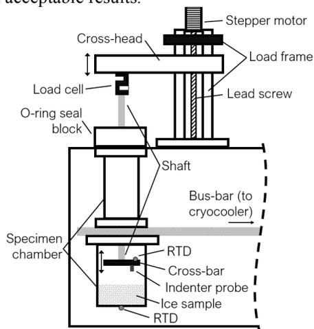
**Figure 1: Schematic representation of instrumented indentation tester and cryostat. The lower specimen chamber is shown in cross-section.**
