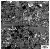
Fig. 2 HAADF-STEM image of the fine-grained matrix of A12169. The matrix is composed of densely packed  $\sim$ 0.5- to  $\sim$ 1- $\mu$ m sized domains containing abundant tiny (typically  $<\sim$ 0.1  $\mu$ m) Fe sulfide. En: enstatite, OI: olivine.
