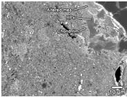
Fig. 1 BSE image of typical fine-grained matrix of A12169. Upper right corner of the image shows that the surface of chondrules experienced aqueous alteration. Thin chondrule rim has a texture different from the fine-grained matrix. mes: mesostasis, HPx: high-Ca pyroxene, Chond: chondrule.
