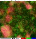
Fig. 4 High-spatial resolution composite pseudo color map of Fe K $\alpha$ , Ni K $\alpha$ , and S K $\alpha$  lines of typical matrix of A12169. There are abundant tiny ( $\sim$ 20 nm) Ni-enriched nanograins.
