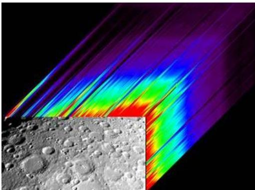
Figure 1. IIRS spectral data cube of a subset image acquired on August 23, 2019. The subset of the image has 169 cross-track samples, 73 lines and 251 spectral channels measuring from 810 to 5026 nm.
