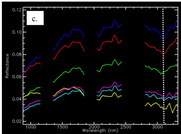
Figure 2. a. Locations of the region of interests (ROIs) in the image and b. corresponding spectral radiance profiles for different surface types such as crater central peak, crater floor, sun-lit inner crater rim and c. spectral reflectance of the corresponding ROIs as shown in a.
