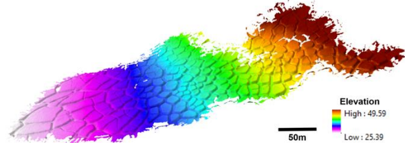
Fig 4. A digital elevation model of a portion of Strand Fiord, Axel Heiberg Island derived from the AkhkaR4DW backpack LiDAR instrument in 3cm resolution.
