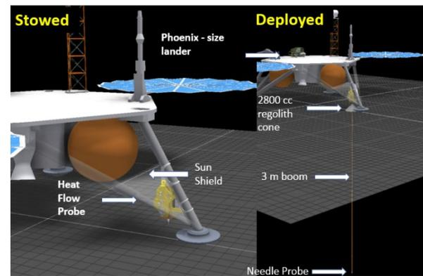
**Figure 1.** A schematic diagram showing LISTER attached to a lander's leg with the probe stowed (left) and deployed (right).
