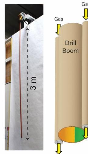
**Figure 4.** Left: the boom of the current prototype fully extended. Right: the new boom design line with thin tubes for gas flow.
