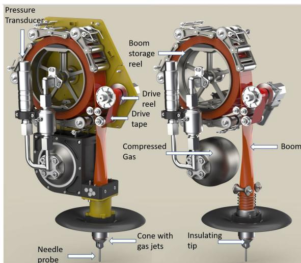
**Figure 2.** Schematics of the deployment mechanism of LISTER.
