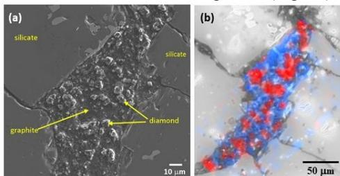
**Fig. 4.** Carbon area in MS-170. (a) SEI. (b) Raman map (red = diamond; blue = graphite).
