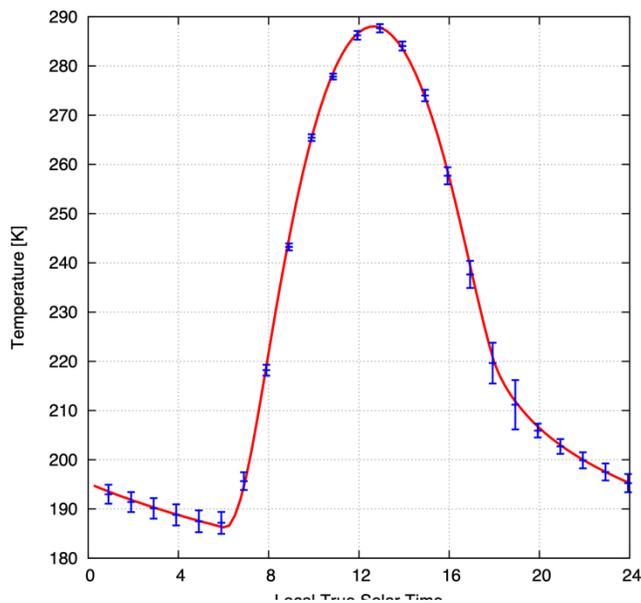
Fig. 2: Example of a diurnal temperature cycle ( $1/24^{\text{th}}$  sol binning) on sol 32. See [3] for error bars discussion. Best, thermal inertia fits is reported in red yielding  $I=190 \pm 10 \text{ J m}^{-2} \text{ K}^{-1} \text{ s}^{-1/2}$  (fits within error bars not shown for clarity). RMS = 0.6 K.
