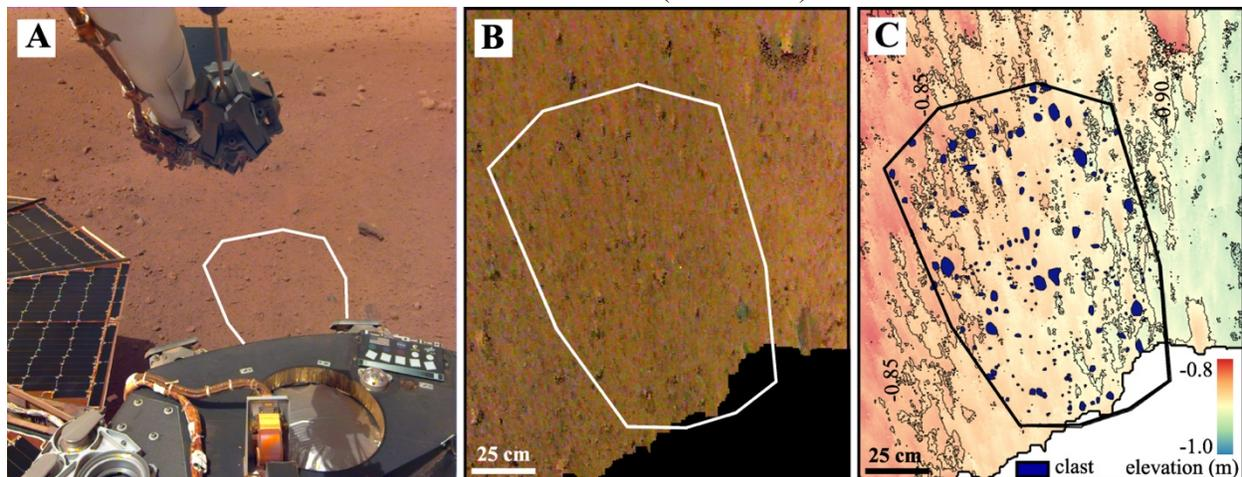
Fig. 1. A: Homestead Hollow looking towards north-northwest, showing parts of the lander deck and solar panels. The white line marks a fraction of the area monitored by the far RAD; B: equirectangular projection of the far RAD spot (5 mm pixel<sup>-1</sup>); C: far RAD spot Digital Elevation Model, accuracy of 1 cm, 5 mm pixel<sup>-1</sup> resolution. 5 cm contour lines, highlighting a tilted surface (~4°) toward the east-southeast. Clasts greater than 1cm are mapped in blue.
