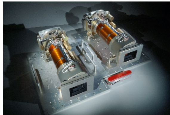
Figure 1. The Mastcam-Z flight cameras. Pocket knife is 89 mm wide, for scale.
