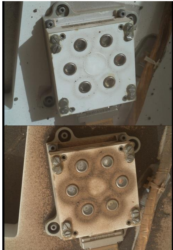
Figure 1. MAHLI images of the REMS UV Sensor approximately at the beginning of the mission (sol 36, top) and more than two Martian Years later (sol 1498, bottom).
