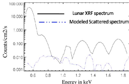
**Figure 5: Lunar X-ray spectrum along with the scattered fraction of the solar spectrum.**
