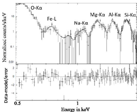
**Figure 4: Lunar X-ray spectra in the imbrium basin region (pixel 2) fitted with a model with lines and scattered continuum.**
