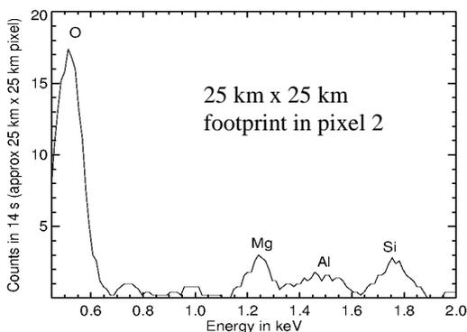
**Figure 3: XRF lines of O, Mg, Al and Si detected from a ground pixel of 25 km x 25 km in the imbrium basin**
