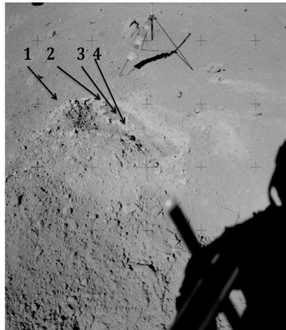
Fig. 2 Apollo 17 Station 3 (EVA-2) trench in rim ejecta of Ballet Crater with indicated location of samples described in Table 1. Long dimension of color chips on gnomon is ~3 cm and gnomon shadow points west northwest. 73001/2 drive tube core site is ~15 m to southwest. (NASA Photo AS17 138 21149)
