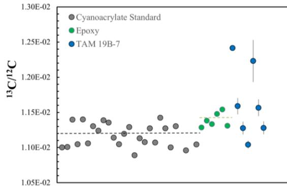
**Figure 2.** Carbon isotope compositions measured in several areas in two fragments in TAM19B-7, along with the cyanoacrylate standard and epoxy in which the fragments were mounted. Two areas on the fragments probably containing carbonate grains show  $^{13}\text{C}$  excesses.  $1\sigma$  error bar = standard error are shown.
