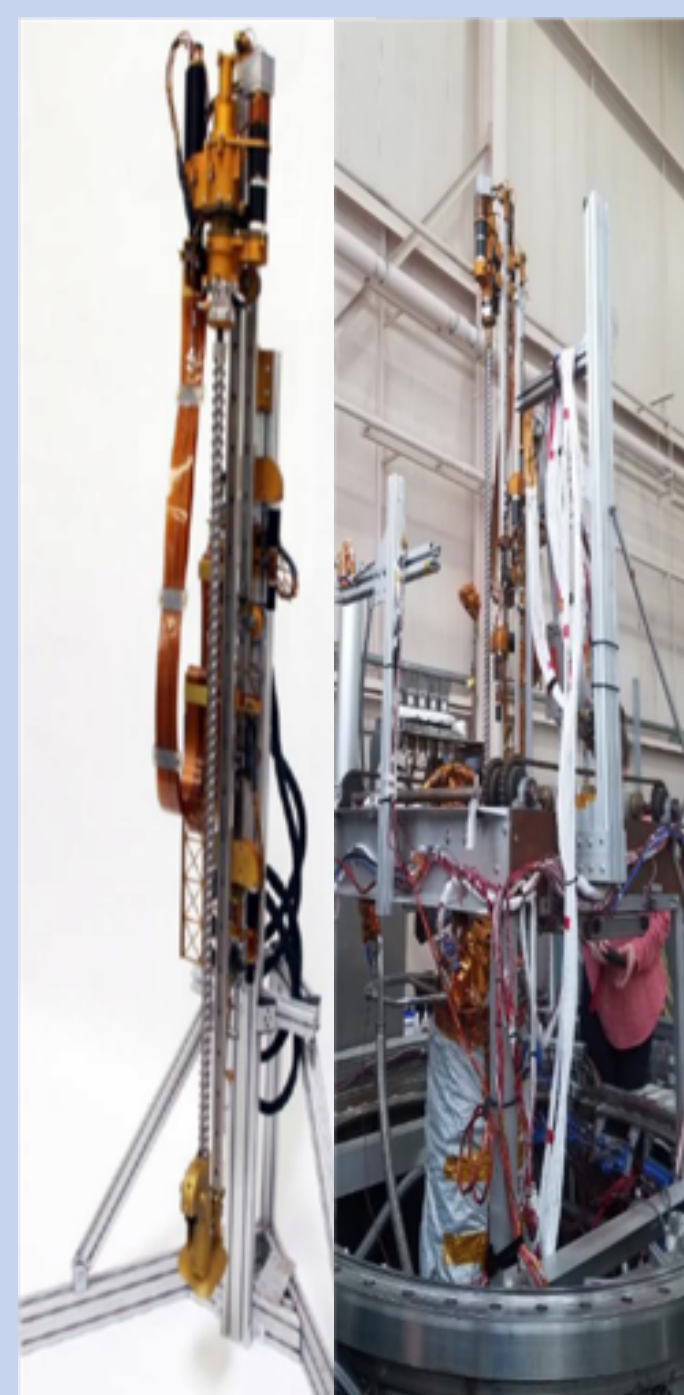
TRIDENT drill undergoing testing in lunar chamber at NASA Glenn.[12]
