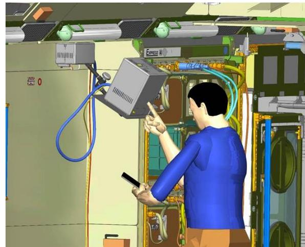
**Figure 3.** Mochii topology in the Japanese Experiment Module within ISS. 95<sup>th</sup> Percentile male user shown operating Mochii with ISS-supplied iPad tablet. Mochii will be powered by 120VAC inverter and connected to station Ethernet and Wifi.
