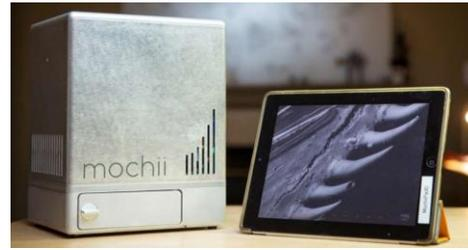
**Figure 1.** Voxa's Mochii™ Electron Microscope (left) with iPad controller (right) with high resolution image of the head of a wheat plant.
