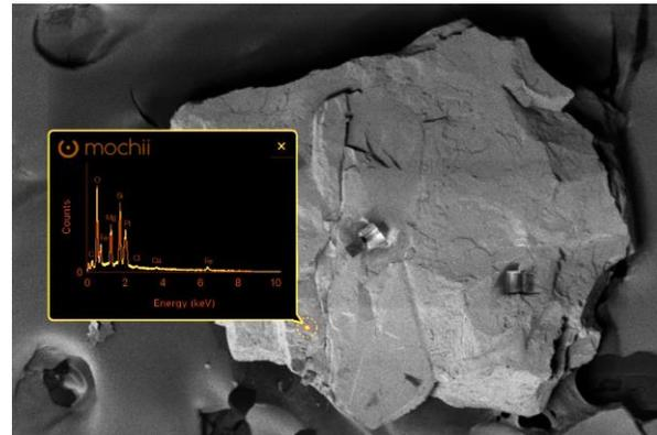
**Figure 2.** Energy-dispersive X-ray (EDS) spectrum acquired with Mochii S on a ~1mm fragment of Martian meteorite Nakhla. Compounds needed to support life have previously been detected on cleaved surfaces of Nakhla.
